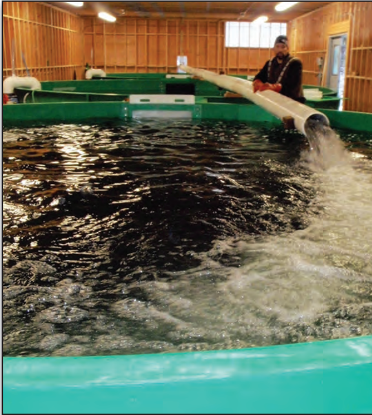
Initial study results show the circular current in the round tanks at the Chiwawa Hatchery is raising healthier steelhead. Photos courtesy of Chelan County PUD.
